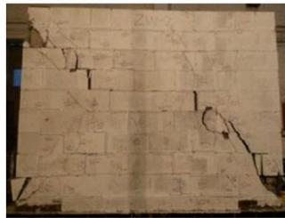
( d ) Test failure of ZW-1
