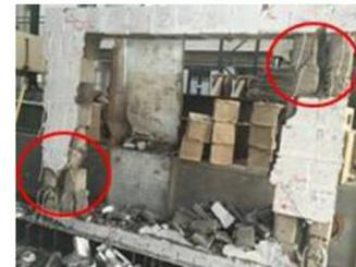
( e ) Failure of built-in structural column and core column in ZW-1
