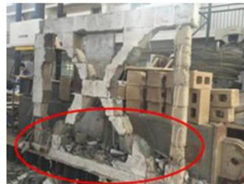
( k ) Failure of built-in structural column and diagonal brace in XCW-1
