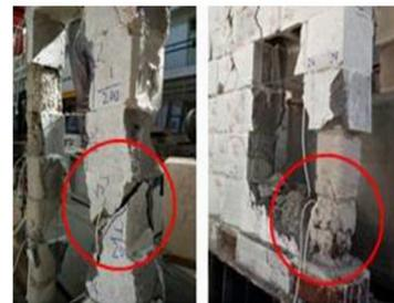
( h ) Failure of built-in structural column and core column in ZW-2
