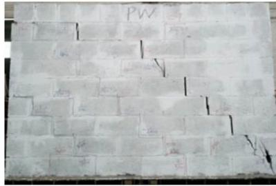
( b ) Test failure of PW
