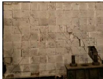
( g ) Test failure of ZW-2
