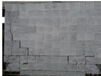
( j ) Test failure of XCW-1
