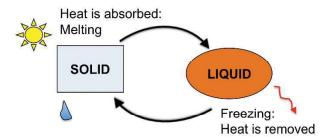
Figure 4.4 Phase-Change Materials Can Act Like Thermal Batteries
