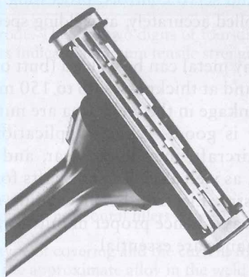
FIGURE 30.16 Detail of Gillette Sensor razor cartridge, showing laser spot welds.
