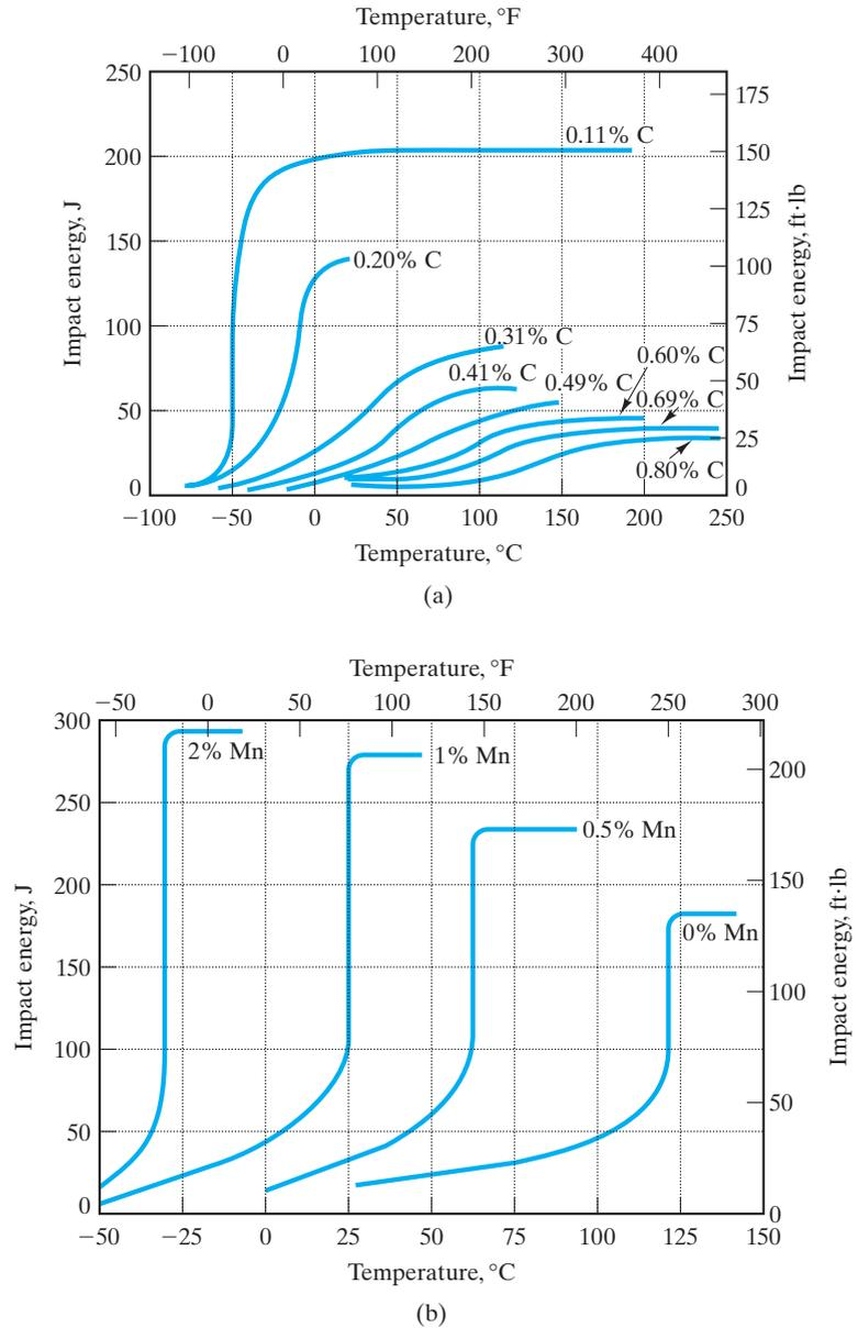
**FIGURE 8.3** Variation in ductile-to-brittle transition temperature with alloy composition. (a) Charpy V-notch impact energy with temperature for plain-carbon steels with various carbon levels (in weight percent). (b) Charpy V-notch impact energy with temperature for Fe-Mn-0.05C alloys with various manganese levels (in weight percent). (From *Metals Handbook, 9th ed., Vol. 1, American Society for Metals, Metals Park, OH, 1978.*)
