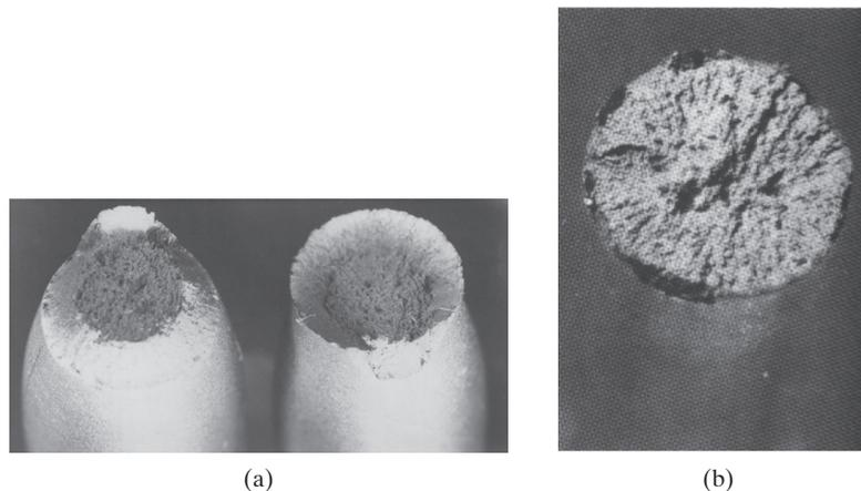
**FIGURE 8.4** (a) Typical “cup and cone” ductile fracture surface. Fracture originates near the center and spreads outward with a dimpled texture. Near the surface, the stress state changes from tension to shear, with fracture continuing at approximately 45°. (From *Metals Handbook, 9th ed., Vol. 12, ASM International, Metals Park, OH, 1987*) (b) Typical cleavage texture of a brittle fracture surface. (From *Metals Handbook, 8th ed., Vol. 9, American Society for Metals, Metals Park, OH, 1974.*)
