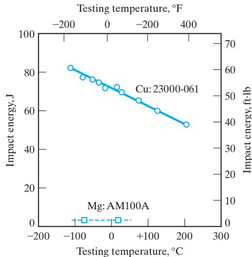
**FIGURE 8.2** Impact energy for a ductile fcc alloy (copper C23000–061, “red brass”) is generally high over a wide temperature range. Conversely, the impact energy for a brittle hcp alloy (magnesium AM100A) is generally low over the same range. (From Metals Handbook, 9th ed., Vol. 2, American Society for Metals, Metals Park, OH, 1979.)
