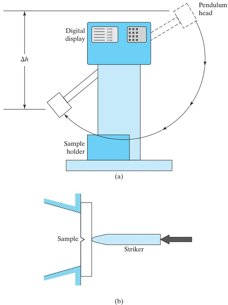
**FIGURE 8.1** (a) Charpy test of impact energy. The drop in height between the initial and final pendulum positions ( $\Delta h$ ) corresponds to the impact energy absorbed by the sample upon fracture. (b) The instant of contact between the Charpy striker (inside the pendulum head) and the sample.
