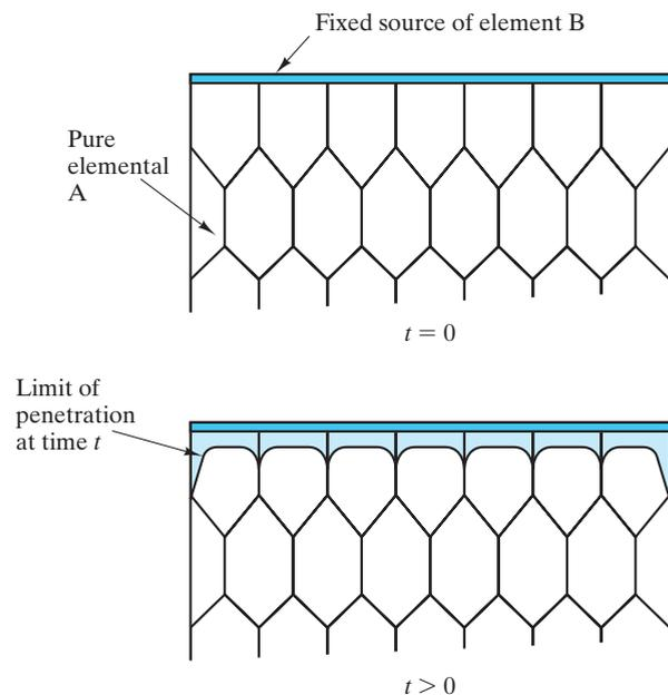
**FIGURE 5.18** Schematic illustration of how a coating of impurity B can penetrate more deeply into grain boundaries and even further along a free surface of polycrystalline A, consistent with the relative values of diffusion coefficients ( $D_{\text{volume}} < D_{\text{grain boundary}} < D_{\text{surface}}$ ).
