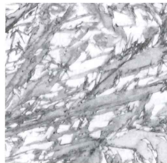
FIGURE 4.13 (a) Hardness of martensite as a function of carbon content. (b) Micrograph of martensite containing 0.8% carbon. The gray platelike regions are martensite; they have the same composition as the original austenite (white regions). Magnification: 1000 \times .
