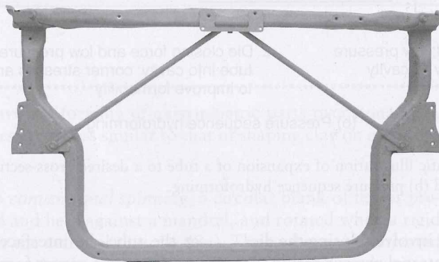
FIGURE 16.44 Hydroformed automotive radiator closure, which serves as a mounting frame for the radiator.
