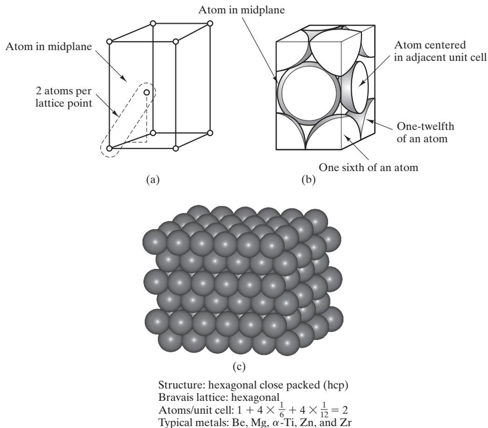
**FIGURE 3.6** Hexagonal close-packed (hcp) structure for metals showing (a) the arrangement of atom centers relative to lattice points for a unit cell. There are two atoms per lattice point (note the outlined example). (b) The actual packing of atoms within the unit cell. Note that the atom in the midplane extends beyond the unit-cell boundaries. (c) The repeating hcp structure, equivalent to many adjacent unit cells. [Part (c) courtesy of Accelrys, Inc.]
