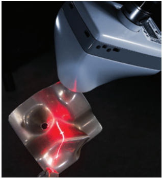
3D scanning helps in controlling products, either with laser or probe measurement. It is also a key technology for the reverse engineering of products, pieces, tools or artifacts
