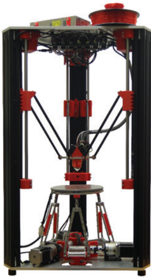
6-axis FDM printer with tiltable bed (developed by IMS)
