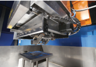
4-axis redundant deposition head designed by SUPSI for the EU project BOREALIS (Advanced Concept of Flexible Machine for Additive and Subtractive Manufacturing, 2015–2017) in which SUPSI also acted as technical coordinator
