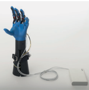
Hand prosthesis manufactured with AM (developed by IMS)
