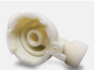
ABS part made with Arburg Freeformer after the water-soluble support structure has been removed
