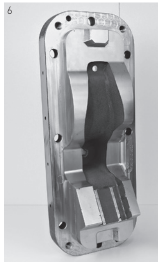
5 and 6 Laser-sintered metal molds for fabrication of EPP foam
