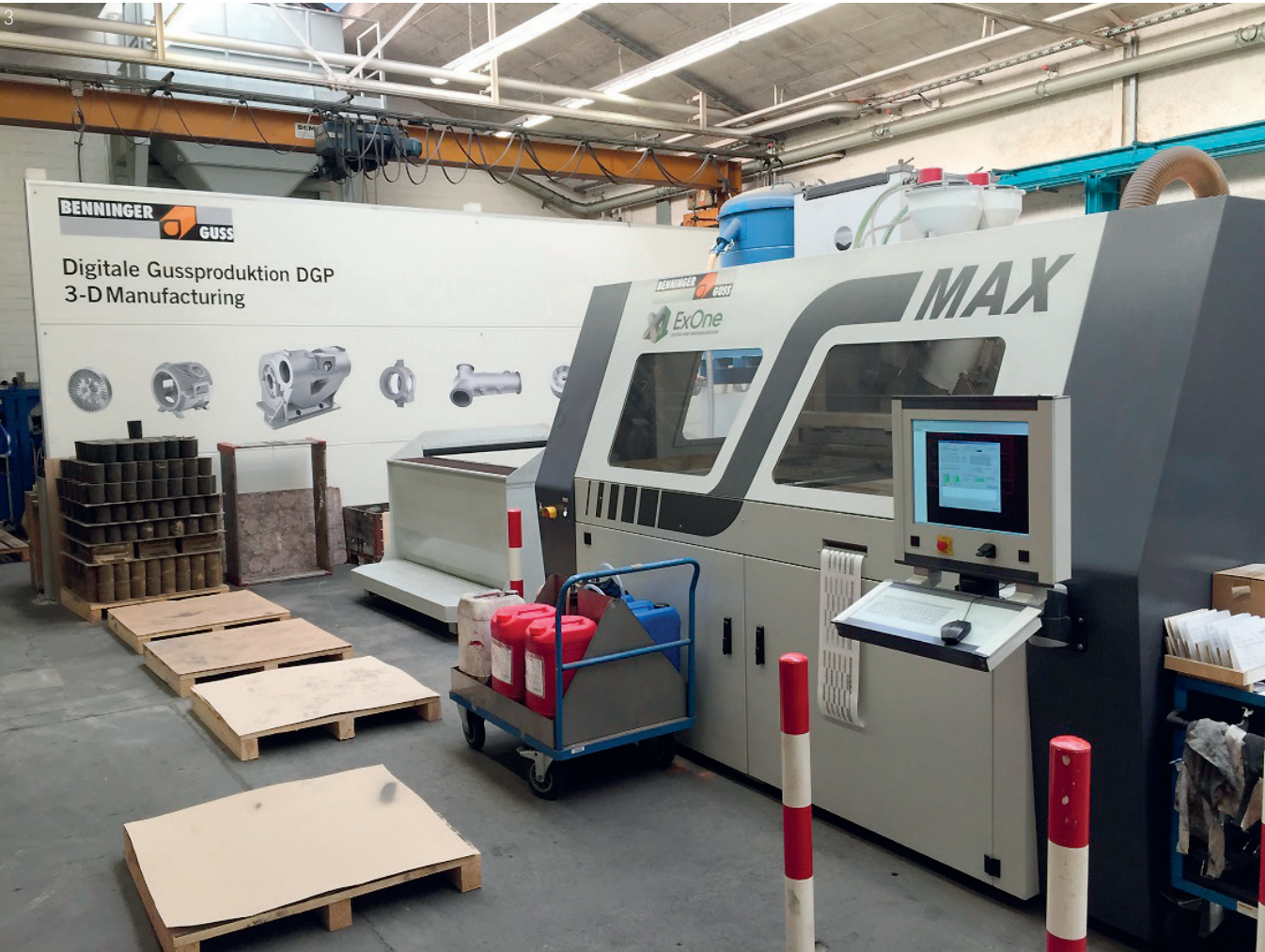
3 ExOne machine used to fabricate sand casting molds through binder jetting
