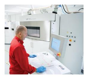
The SLS process begins with heating up a bin of polymer powder to a temperature just below the melting point of the material. A recoating blade or roller then deposits a very thin layer of powder - typically 0.1 mm thick - onto the build platform.
