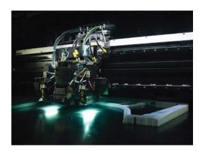
Material Jetting works in a similar way to standard inkjet printing. However, instead of printing a single layer of ink on a piece of paper, multiple layers of material are deposited upon each other to create a solid part. Multiple print heads jet hundreds of tiny droplets of photopolymer onto the build platform, which are then solidified (cured) by the UV light source.
