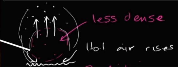
Combustion reaction creates energy: kinetic energy is transferred to neighbouring molecules by collisions
