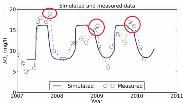
**Figure 6** | Measured and observed sulphate concentrations in ATEs well W10 with screen between –50 and –52 m MSL over the period 2007–2010. The circles show the second breakthrough of ATEs water from the adjacent ATEs well (see text for further description).
