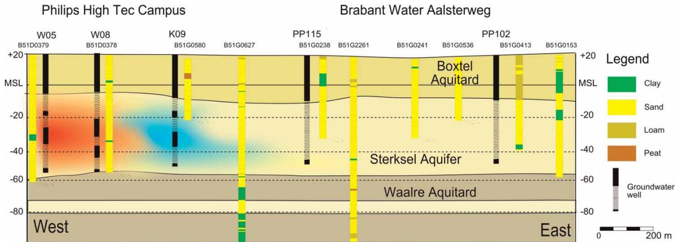
**Figure 2** | Hydrogeological cross section of the ATEs study site in Eindhoven. Aalsterweg is a PSWF of water supply company Brabant Water. PP = pumping well of PSWF; W05, W08 and K09 are part of the ATEs system and simulated in the Modflow-MT3DMS model.
