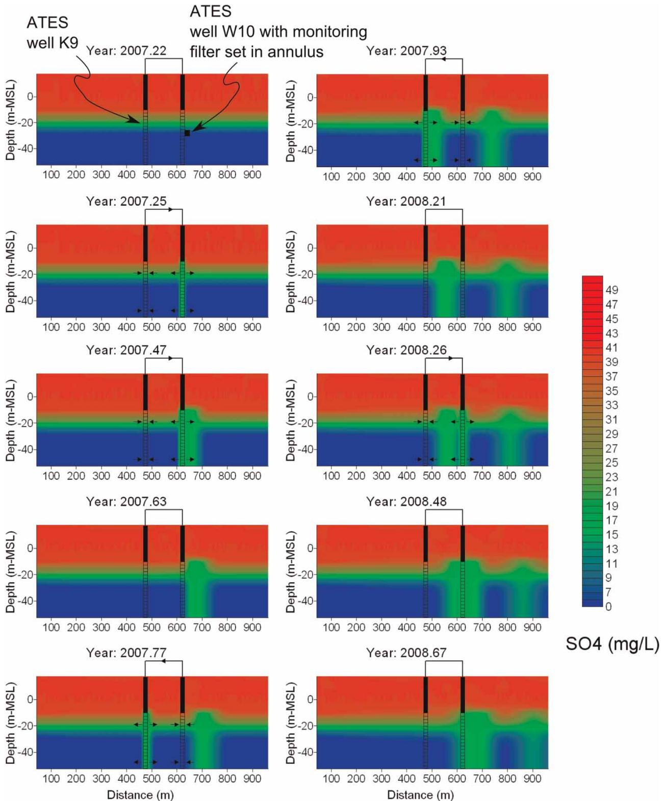
**Figure 5** | Simulated sulphate concentrations (shading) during several periods over the 3 year simulation period. Two ATEs wells (K9 and W10) are shown, top left panel shows location of the monitoring screen set in the annulus of W10. The observed and simulated SO<sub>4</sub> concentrations for this monitoring screen are shown in Figure 6.
