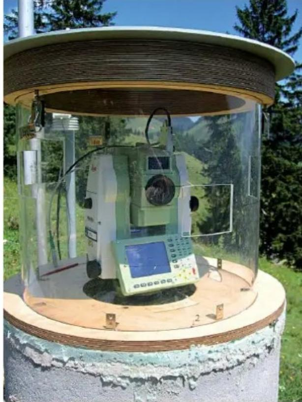
*Fig. 6. The IATS prototype in its housing at the test site
