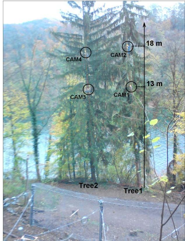
Figure 6. The four cameras are fixed on two trees at 13 meters and 18 meters height, respectively.
