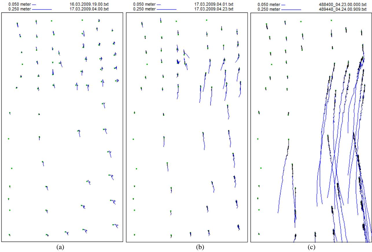
Figure 15. Horizontal displacement of the tennis balls, (a) 1 fph between 6:00 pm and 3:00 am, (b) 1 fpm between 3:01 am and 3:23 am, and (c) 5 fps between 3:23:00 am and 3:24:00 am.
