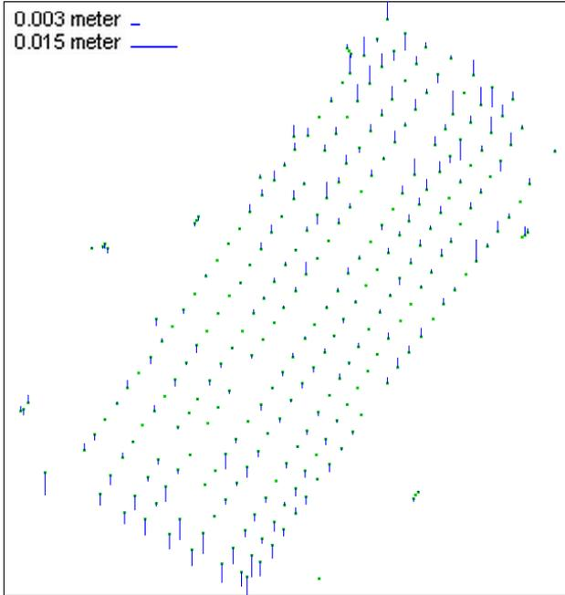
Figure 10. The vertical displacements between the 28.10 and 29.10 epochs. Upward arrows show rising and downward arrows show lowering points.
