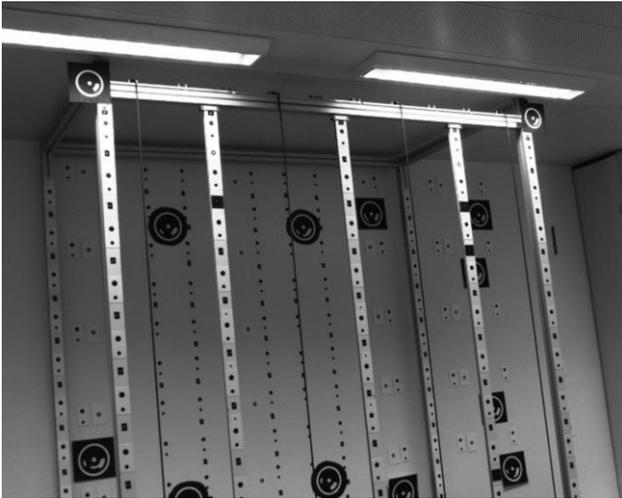
Figure 12. The photogrammetric 3D calibration field at the Institute of Geodesy and Photogrammetry at ETH Zurich.
