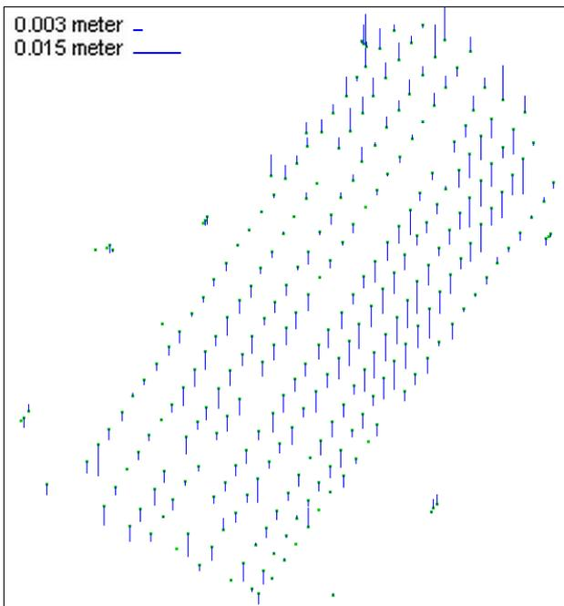
Figure 11. The vertical displacements between the 28.10 and 31.10 epochs.
