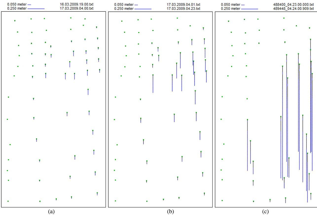
Figure 16. Vertical displacement of the tennis balls in the same timeframes as Figure 15, (a) 1 fph, (b) 1 fpm, and (c) 5 fps.
