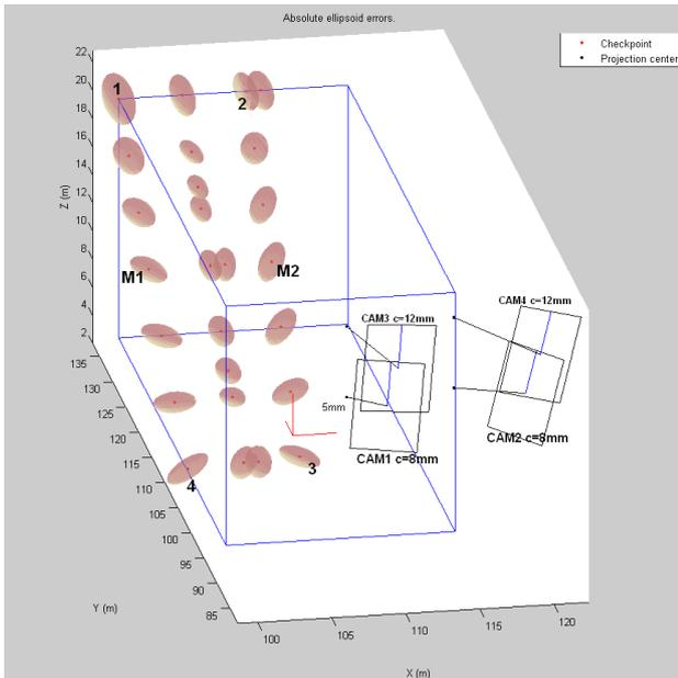
Figure 5. The a priori estimated error ellipsoids of some representative signalized targets.
